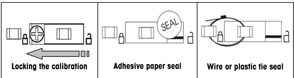
Figure 4-1. Locking and Sealing the Calibration Lock Switch.
