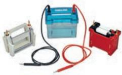
213714 Western Blot/Nucleic Acid Transfer Apparatus
