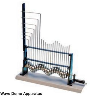
Make waves with this affordable apparatus that demonstrates both longitudinal and transverse waves. The plastic highlighted tips provide easy observation of wave motion. The rotating handle is equipped with a circular scale marked in degrees to indicate rotation. Includes instructions.
