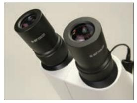
High eye point eyepieces allow spectacle wearers access to the complete field of view
