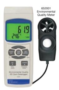
probe (also accepts standard type K or J thermocouple probe), 6 AA batteries, 2-GB SD card, instruction manual, and 5-year warranty.
