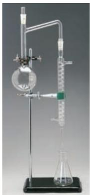
725634 Distillation/Distilling Apparatus
