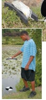
652262 Secchi Disk with Calibrated Line
