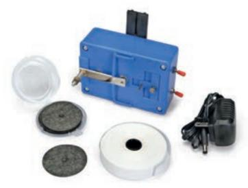
751375 Recording Timer, 751374 Carbon Discs, and 751378 Recording Tape
