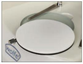
Black-and-white stage plate is included for increased contrast of opaque specimens
